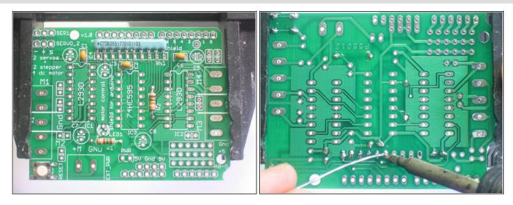
Step 4 — Solder the reset switch and resistor network.
